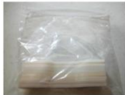
Fig 5. Specimens for water absorption sealed in a plastic bag.
