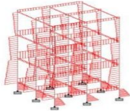
Fig 17. Bending of Structure.
