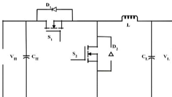
Fig 4. Circuit diagram of the buck-boost converter.
