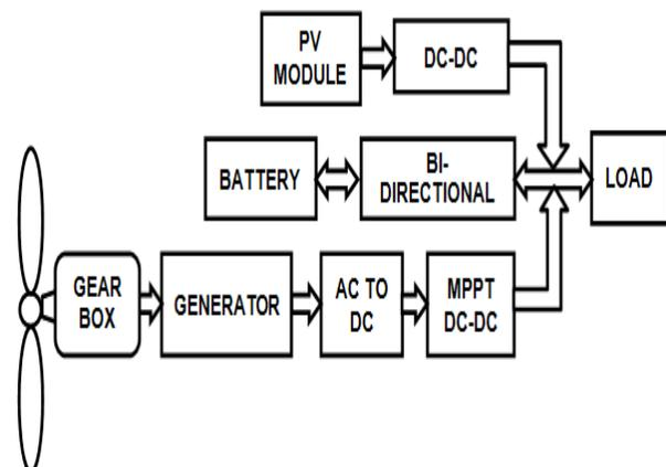
Fig 1. Architecture of hybrid system.
