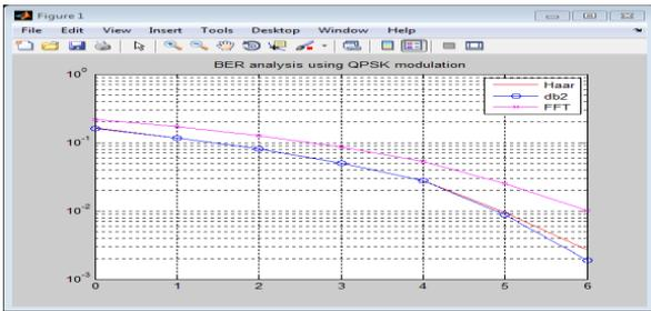
Fig 2: BER using QPSK Modulation.
