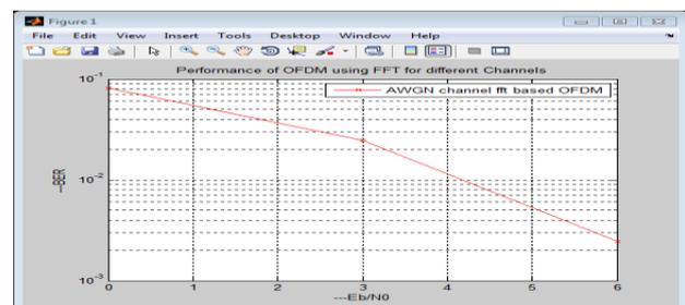
Fig 1: BER of Conventional OFDM using FFT.
