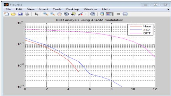
Fig 3: BER vs SNR using 4-QAM.
