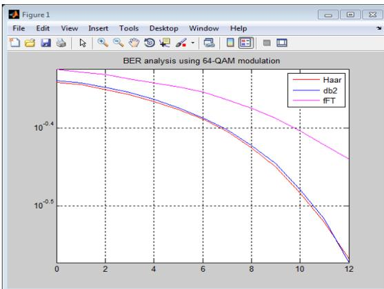
Fig 5: BER vs SNR using 64-QAM
