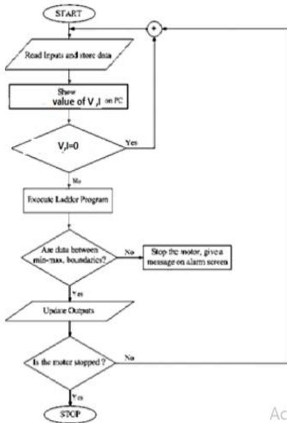
Fig 4. Flow Chart of the Program of Software developed.
