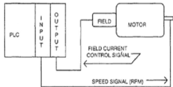
Fig 3. Control System for PLC and Motor.
