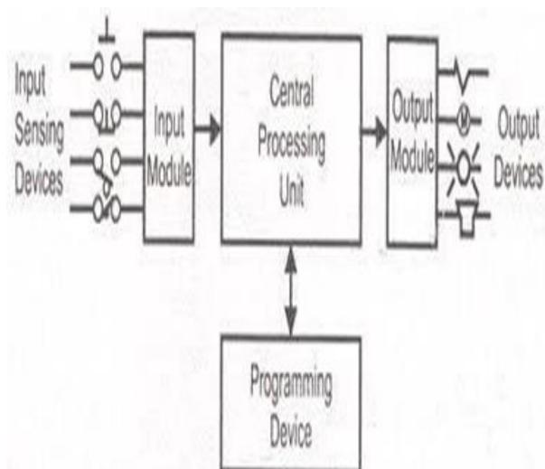
Fig 1. General structure of PLC.
