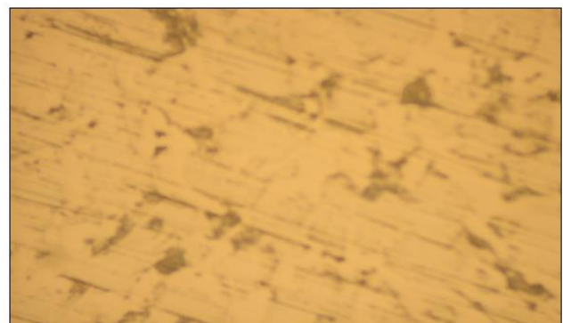
Fig 3. Micrograph of Nodular Graphite.
