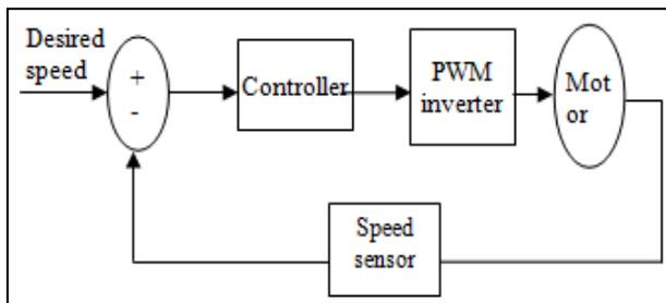
Fig 1. General controller for induction motor. [13]
