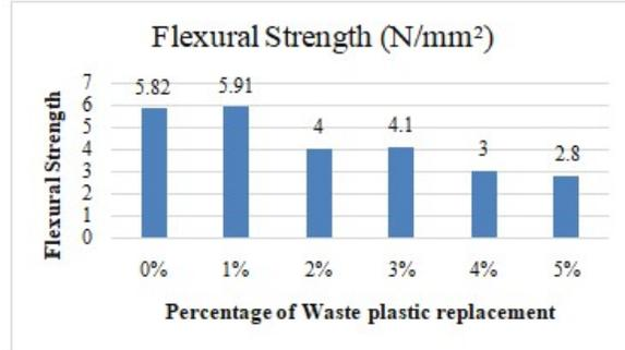
Fig 3. Flexural Strength at 28 Days.
