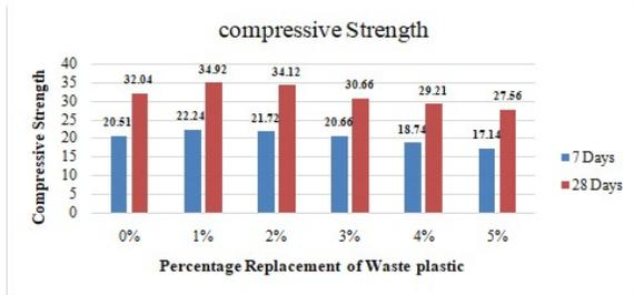
Fig 2. Compressive Strength of Concrete M25.
