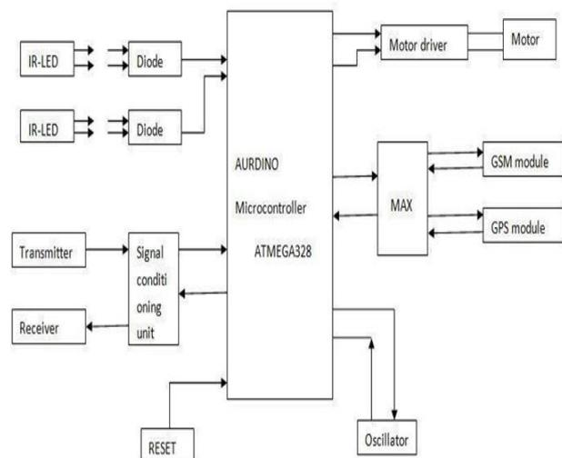
Fig 1. Block Diagram of Testing Vehicle.
