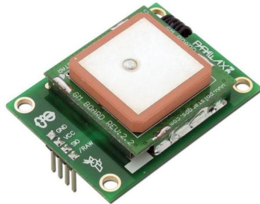
Fig 2. GPS navigation device.
