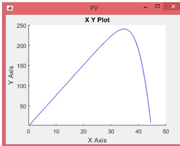
Fig 11. PV Characteristics Waveform.
