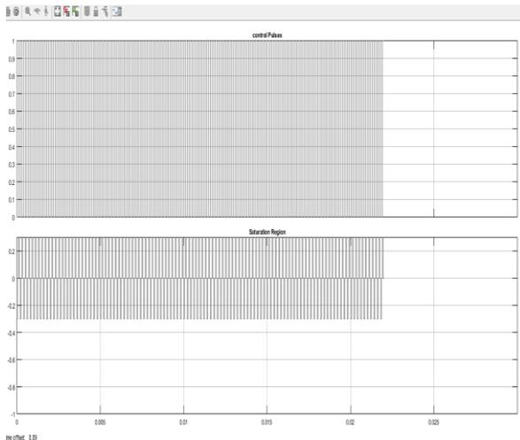
Fig 14. Solar Panel DC-DC Boost Converter Pulses.
