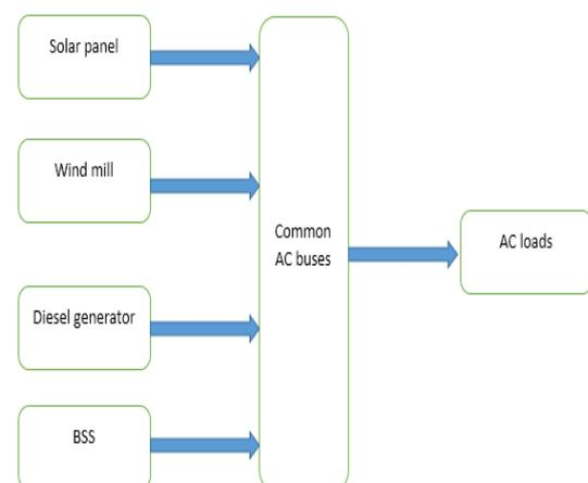
Fig 1. Proposed Integrated Energy System.
