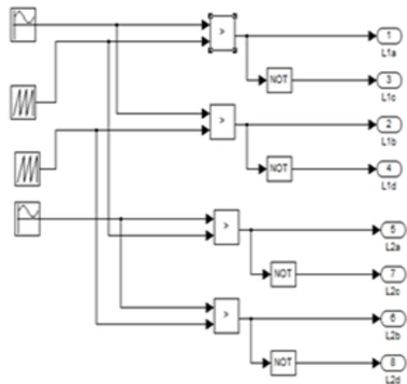
Fig 5. Simulink model of switching pulses of converter system.
