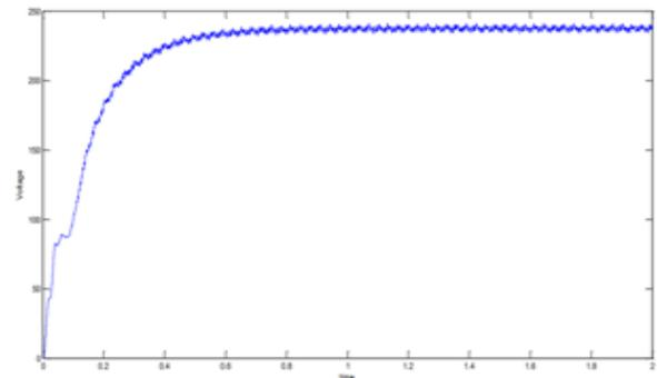
Fig 9. Output voltage of Boost converter.
