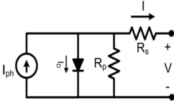
Fig 2. Simplified PV cell model.
