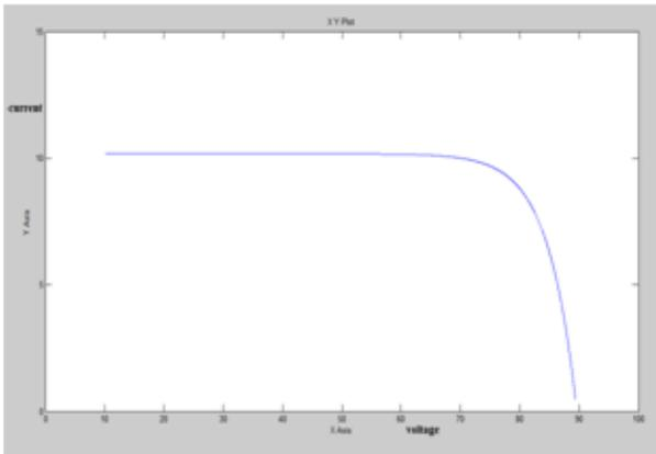
Fig 6. Characteristic solar PV panel.
