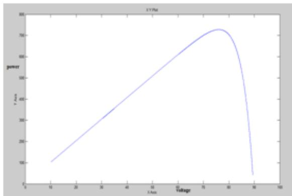
Fig 7. PV Characteristic solar PV panel.
