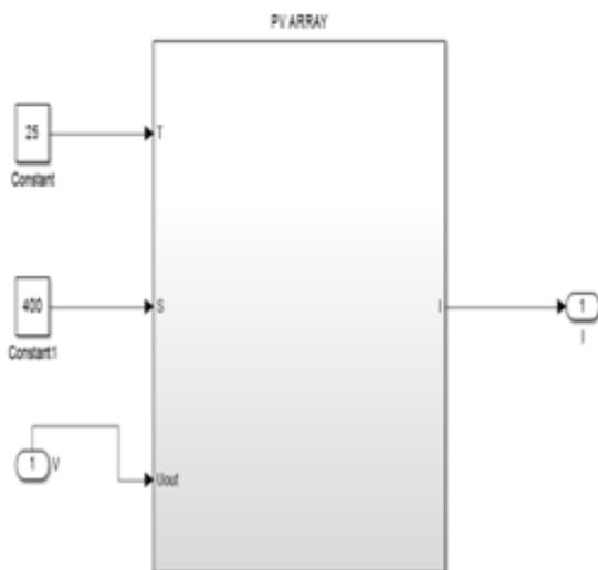
Fig 3. Masked block diagram of the modeled solar PV panel.
