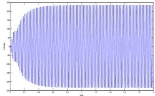
Fig 10. Output voltage of inverter.
