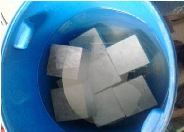
Fig 3. Curing of cubes and beams.
