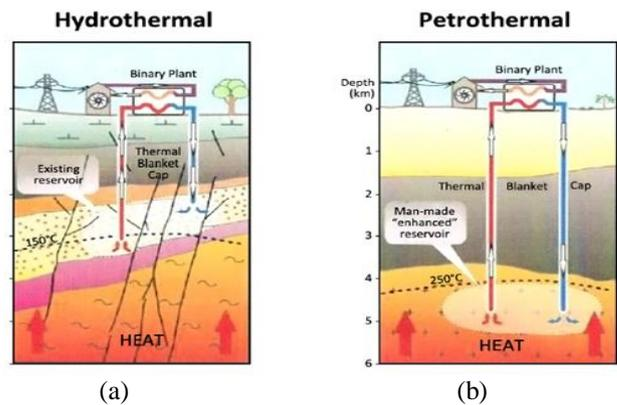
Fig 2: (a) Heat carrier (i.e steam/ Hot water) at locally present Depth-very rare (Energies, 2014)
