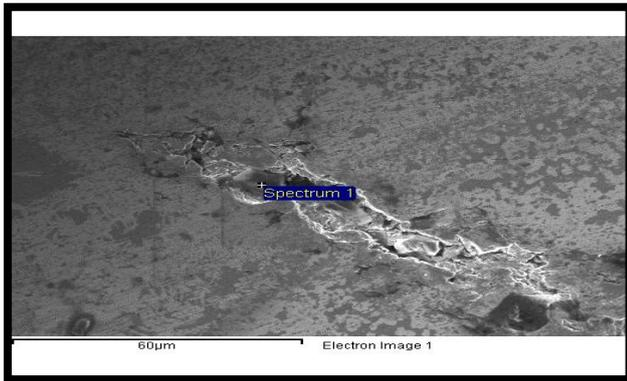
Fig.5 (b) Compositions of the crack portion identified using energy dispersive spectroscopy.
