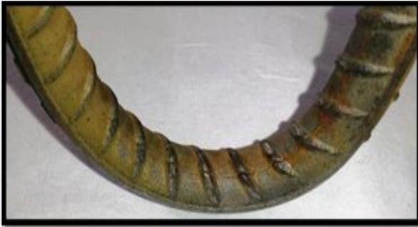
Fig 1. 8mm TMT Bar cracked during bending of operation on the transverse rib.
