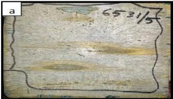
Fig 2. (a) Image of billet samples showing blow holes (b) Image of billet samples showing blow piping defect in the center of the sample.
