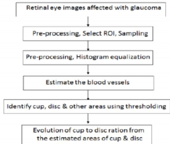
Fig 4. Block Diagram
