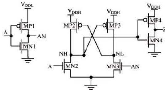
Fig. 1 Conventional DCVS level converter [16]
