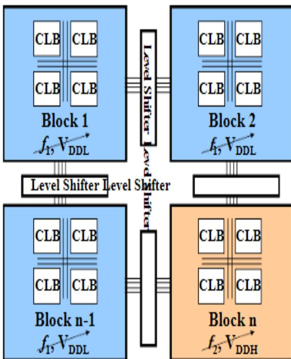
Figure 4 Block-level VDD-hopping.
