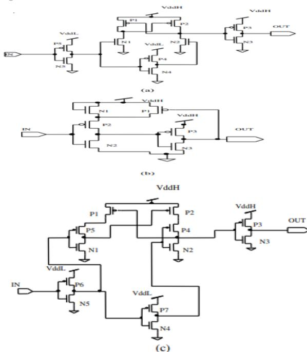
Figure.2. Level shifter circuits (a) Conventional (b) Single supply (c) Contention mitigated.
