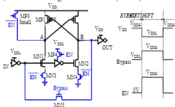
Figure 6 Bypassing enabled level shifter (BELS).
