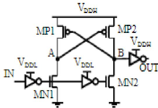
Figure 5. (a) Conventional level shifter.
