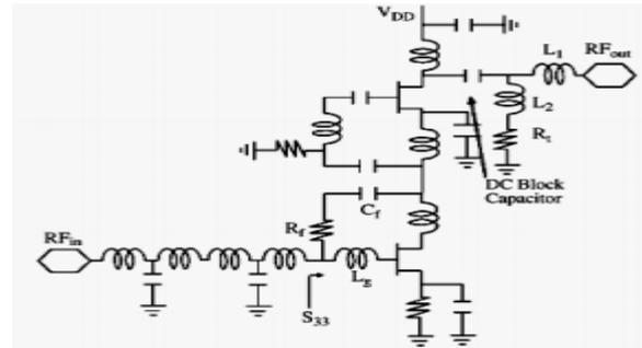
Fig. 2. Simplified schematic of the wideband LNA [4].
