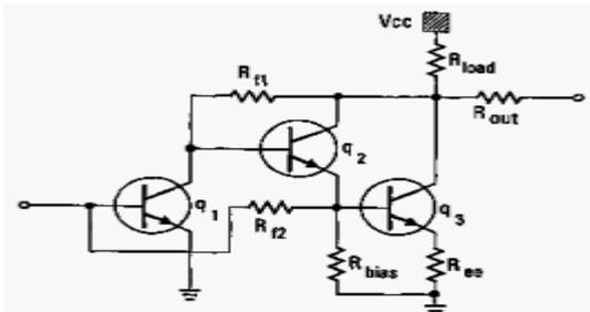
Fig. 1. Schematic of the direct-coupled HBT amplifier [3].
