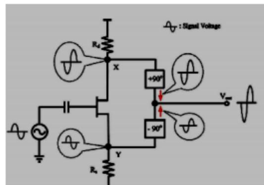
Fig. 3 Illustration of forward combining technique [5].
