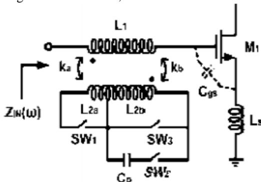
Fig 4 Multimode LNA with a reconfigurable multi-tap transformer as the gate inductor [6].
