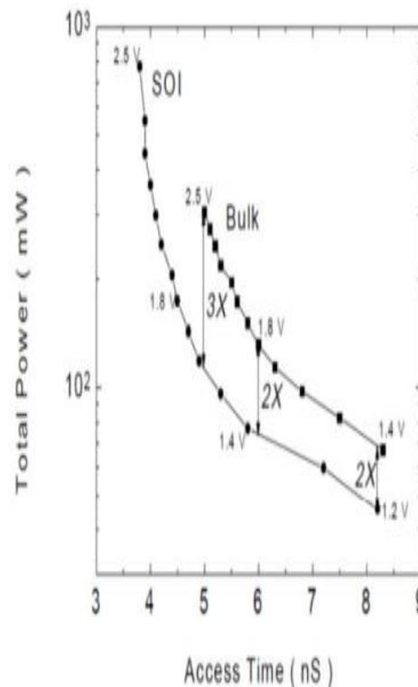
Fig.2.Improvement in execution time by using SOI
