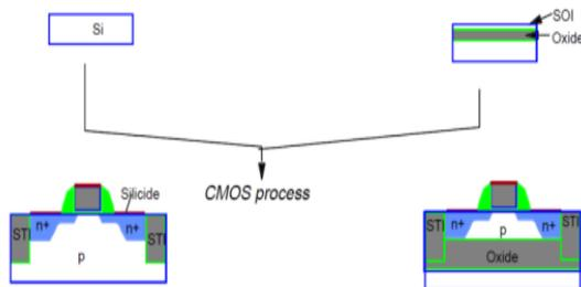
Fig.3. comparison between SOI and bulk CMOS
