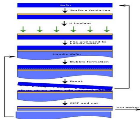
Fig. 1. Fabrication of silicon on insulator through oxidation.
