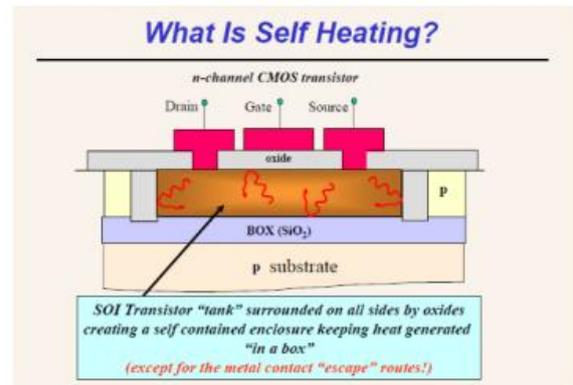
Fig.4. Self heating effect in SOI transistor.
