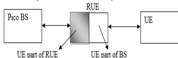
Figure 2 Relay UE Composition and Connection Model.
