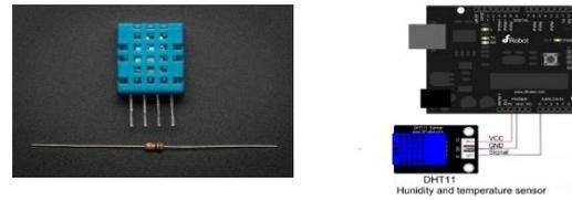
Fig. DHT11 basic Temperature and Humidity Sensor.
