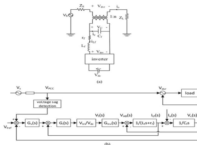
In Figure 1 , VSVS is the system voltage, VdvrVdvr is the output voltage of DVR setup. VrefVref is the instruction voltage. GV(s)GV(s) is the controller of voltage outer loop, Gi(s)Gi(s) is the controller of current inner loop, Vtri/VdcVtri/Vdc is the voltage transformation, Ginv(s)Ginv(s) is the inverter bridge modulation model which is in relationship with Vdc/VtriVdc/Vtri.
