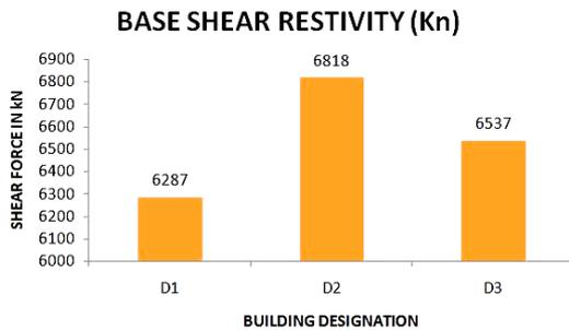
Fig 5: Base shear resistivity (kN) for story 7 for load comb. 1.2(DL+LL+EE)
