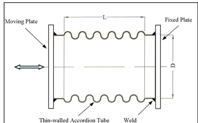
Fig. 1: Schematic view of Accordion Metallic Damper (AMD) source reference no 4.
