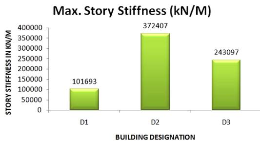
Fig 6: Story Stiffness (kN/M) for story-7 for load comb. 1.2(DL+LL+EE)
