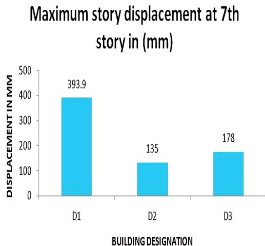
Fig 4: Max story displacement for story 7 for load comb. 1.2(DL+LL+EE)
