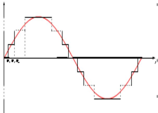
Fig 2. Generalized Stepped Waveform of MLI.
