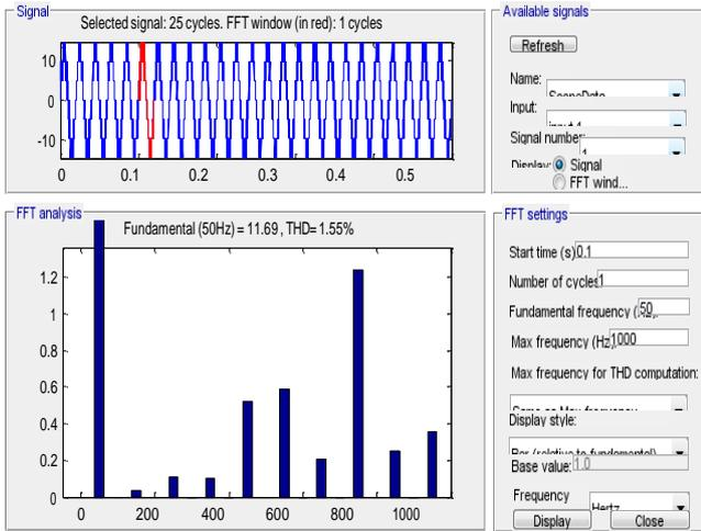
Fig 6. FFT Analysis of current of proposed work with Resistive load.
