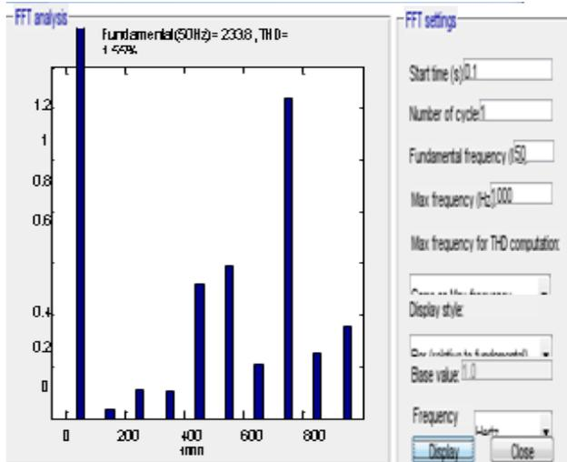
Fig 8. FFT analysis of voltage of resistive load.
