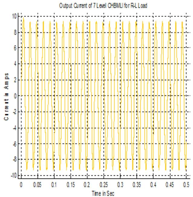
Fig.9. Current Behavior of R-L Load in proposed CHBMLI.
