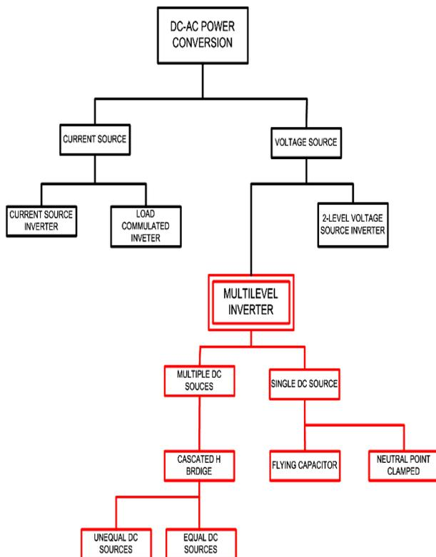
Fig.1. Classification of multilevel inverter.
