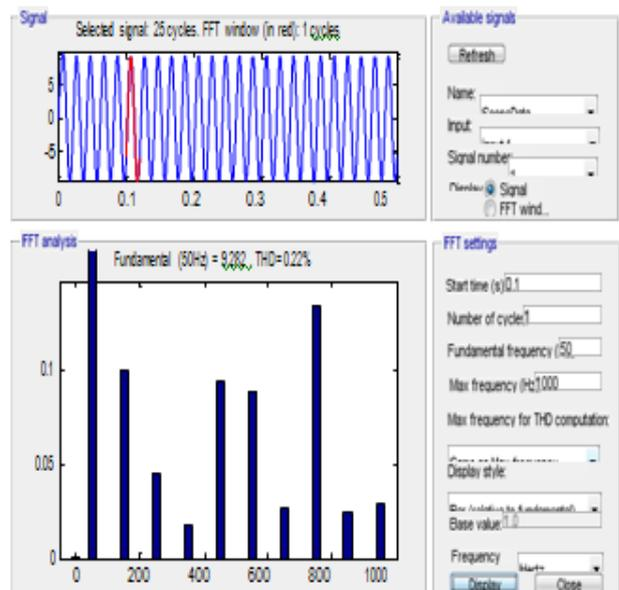
Fig 10. FFT analysis of current of R-L Load
