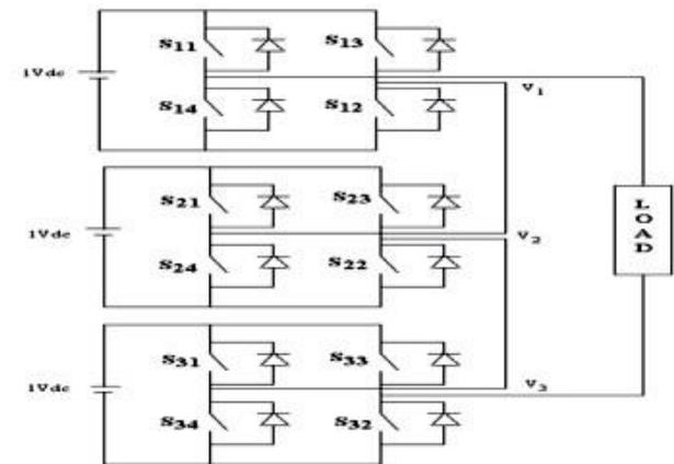
Fig 3: Schematic Diagram of Proposed 7 Level CHBMLI.
