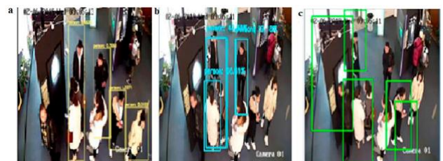
Fig. 8. Detect People by Different Algorithms: (a) Represent results of YOLO-tiny,(b) SSD, and (c) HOG Algorithm.
