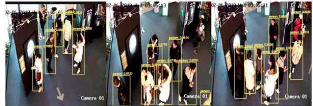
Fig.7. The Results of People Detection Based on YOLOv3 Algorithm.
