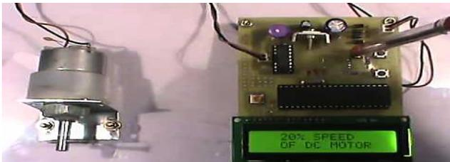
Fig. 4. DC Gear Motor Interface with Controller.
