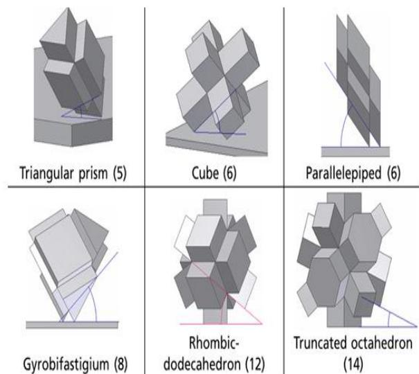
Fig. 4. Basic cell geometries for structure design.
