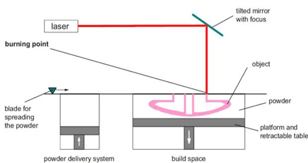
Fig. 2. Schematic diagram of the Selective Laser Melting (SLM) powder-bed process.
