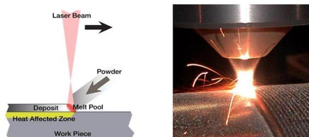
Fig. 3. Schematic of the laser cladding process (Courtesy Sulzer Ltd) and the laser cladding process in action (right).
