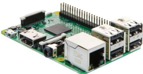
Fig 2 Raspberry pi board.
