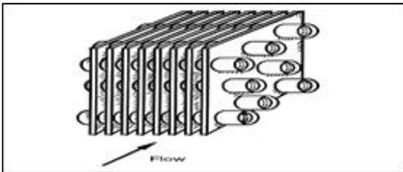
Figure 1. Finned tube heat exchanger.
