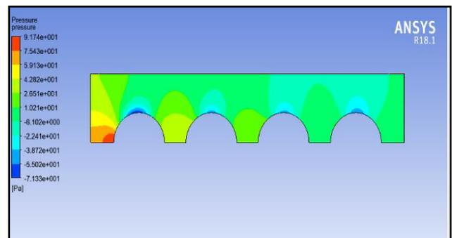
Fig 12. Pressure Contour for ZnO / water .02.
