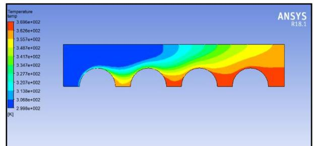
Fig 11. Temperature Contour for ZnO / water .02.
