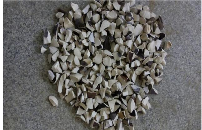
Fig-1 Ceramic waste after crushing to 20 mm down size.
