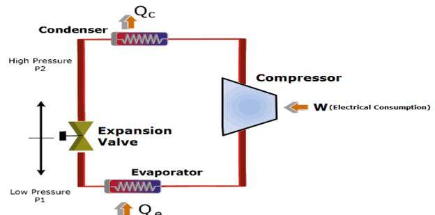
Figure 2 Vapor Compression Refrigeration Cycle.
