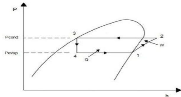
Figure 3 Ideal Vapour Compression Refrigeration Cycle in P-H Diagram.
