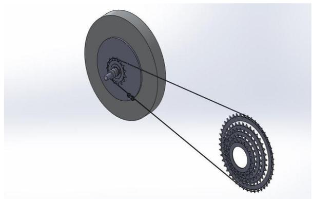
Fig.14. Isometric view of the KERS [2]
