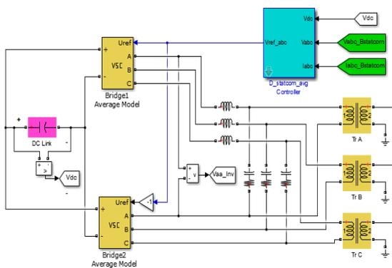
Fig.2 Subsystem of STATCOM.
