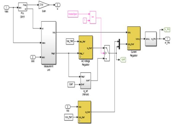
Fig.3 Subsystem of power compensation block.
