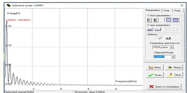
Figure 10 Shows the Fast Fourier Transform of pmos\_carry of 1-Bit Proposed FA.
