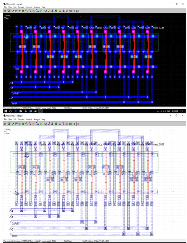
Figure 5 Layout of Proposed 1-Bit Full Adder Design in Micro-wind (90 nm).
