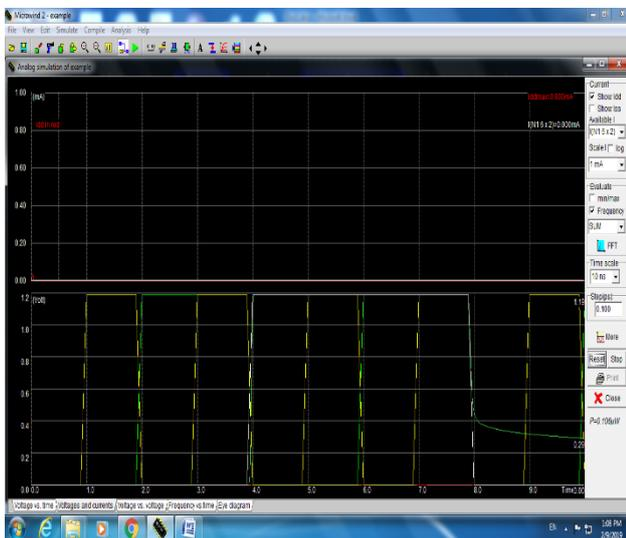
Figure 7 Results Waveform Voltage Vs Current of 1-Bit Proposed FA (90 nm).
