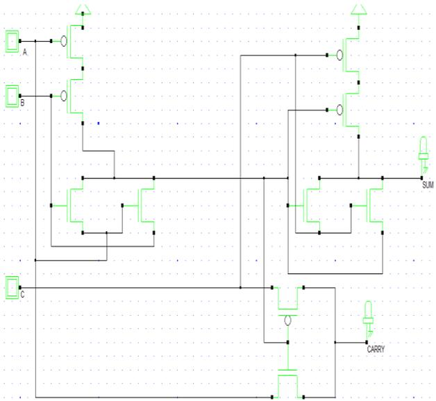
Figure 2 Architecture Design of 1-bit Full Adder using ten transistors
