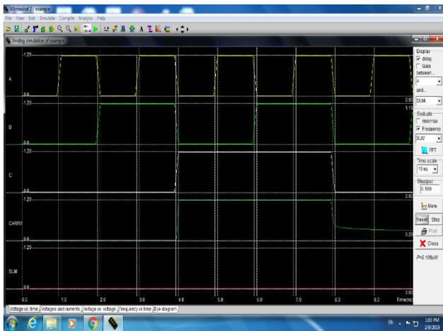
Figure 6 Results Waveform Voltage Vs Time of 1-Bit Proposed FA (90 nm).
