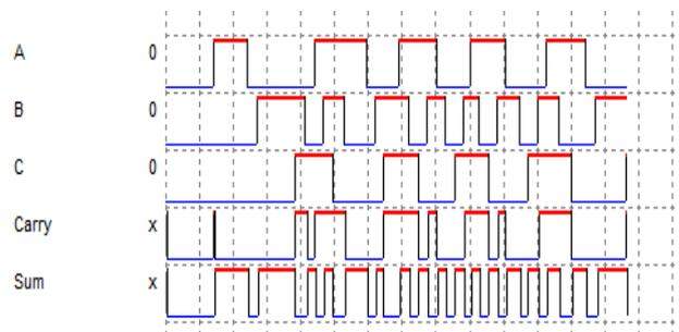
Figure 4 Timing Diagram of DSCH Full Adder Design Micro-Wind Result [(Proposed Design)]
