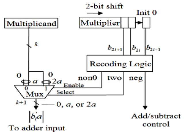
Figure 1 an iterative multiplier structure based radix-4
