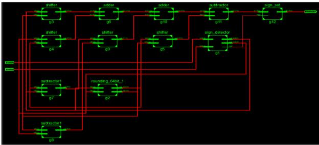
Figure 3 RTL of ROBA Multiplier.
