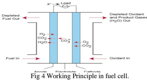
Fig 4 Working Principle in fuel cell.
