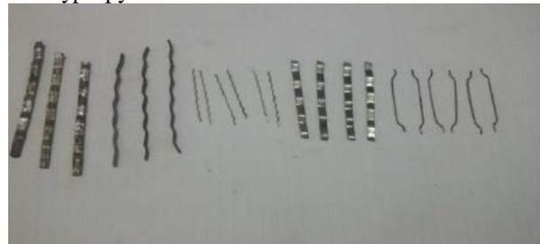
Fig. 2 Different types of Steel Fibres.
