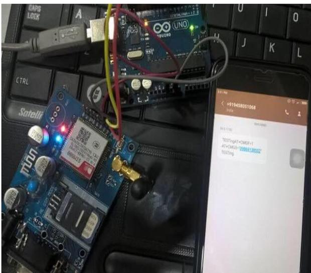
Fig. 3 Interfacing of GSM with Arduino.
