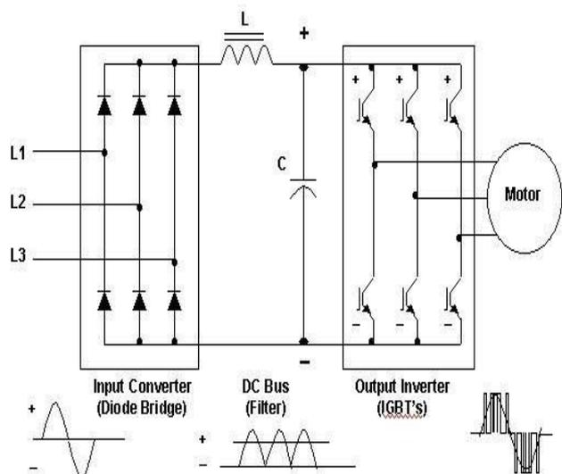
Fig. 1 Basic VFD.
