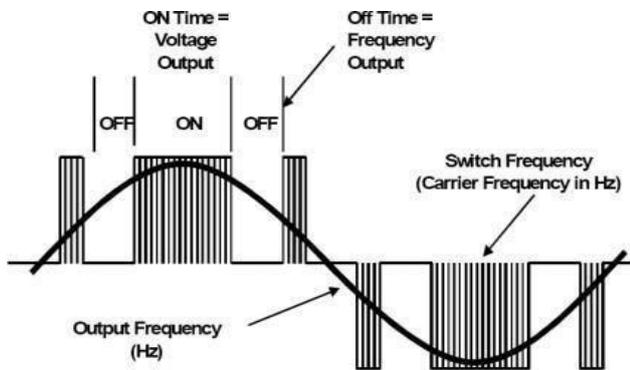
Fig. 2 Drive Output waveform.
