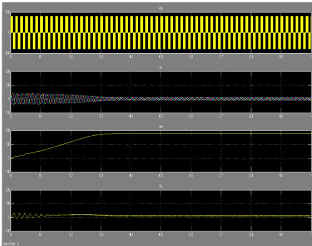
Fig.5 Simulation Graph of Voltage, Current, Speed and Torque of the Asynchronous Motor.
