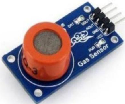
Fig.2 MQ3 Alcohol Sensor Specifications.
