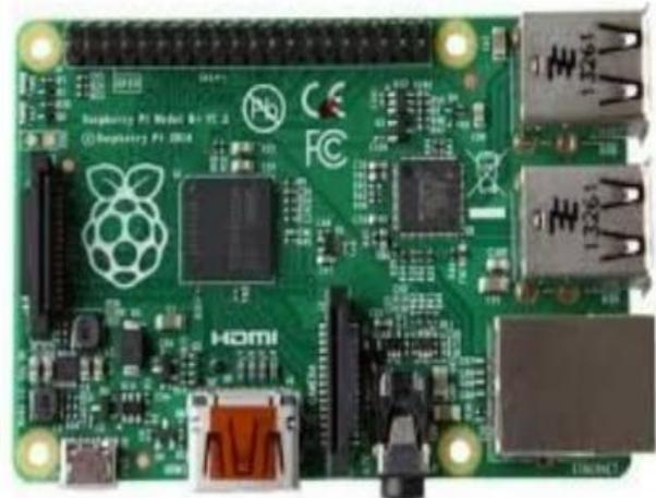
Fig.1 Raspberry Pi Model B V1.1.
