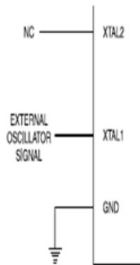
Fig 3 Oscillator Connections.
