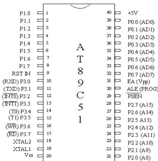
Fig.2 Pin diagram of AT89C51.
