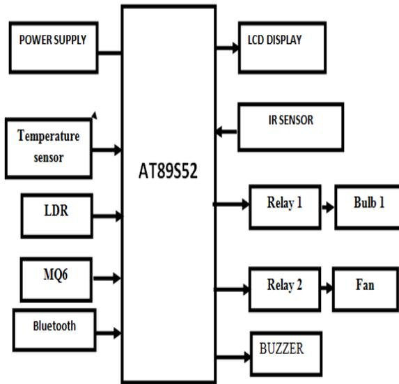
Fig.1 Block Diagram of Automated Energy Saving and Safety System.
