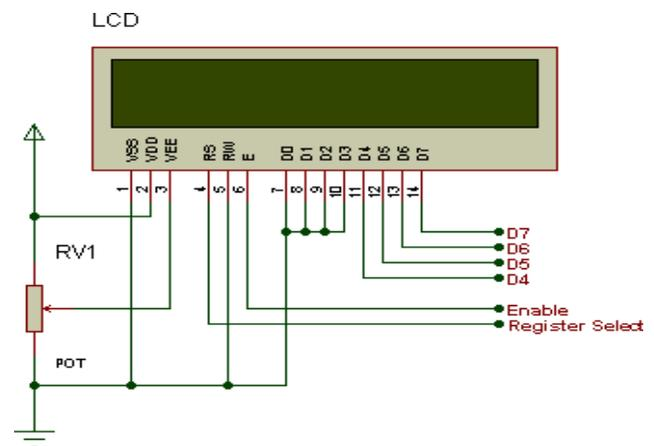
Fig. 5 LCD Pin diagram.
