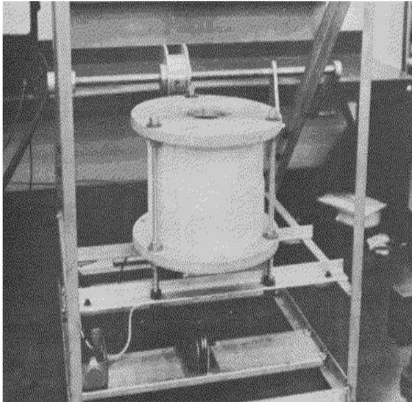
Fig 6 Furnace for applying an aluminum coating to a steel wire.
