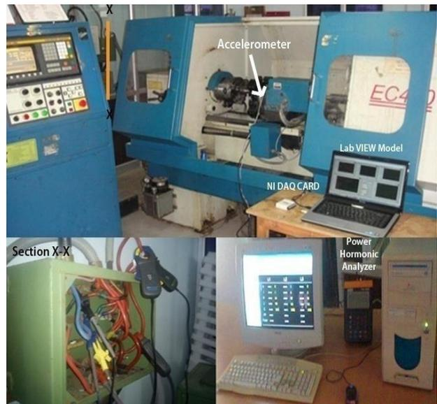
Fig 15 Photographic view of the experimental setup.
