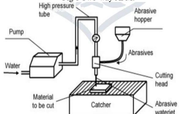
Fig 2 Schematic view of the Abrasive Water Jet Machining process.
