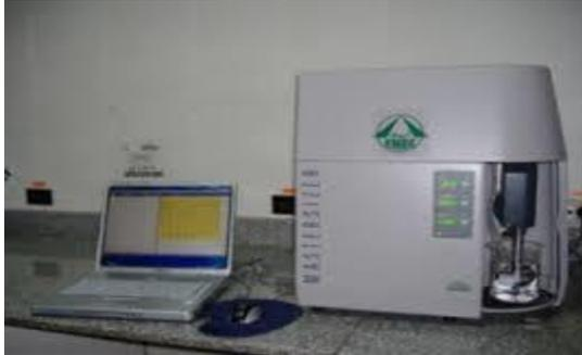
Fig13 Particle size analyzer.
