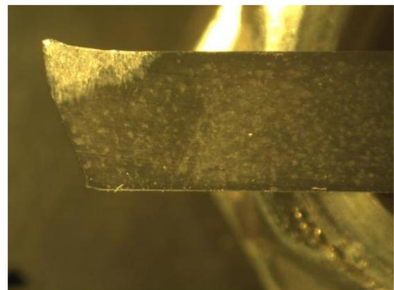
Fig 9 Side wear of the cutting tool.
