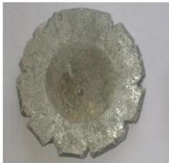
Fig 16 20% by weight reinforced composite after the compression test.
