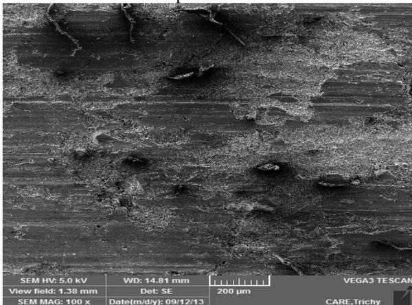
Fig 18 Worn surface of red mud reinforced aluminum matrix with optimal fit.
