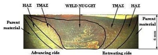
Fig 5 Different zones in the FS welded part.
