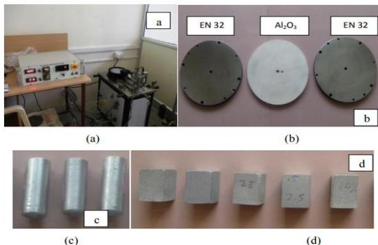
Fig14 (ad) (a) Pin-on-disk device (b) disc material (c) spindle sample (stirring form)(d) cube sample (powder metallurgy).
