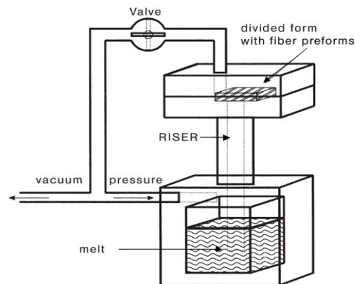
Fig 4 Infiltration technique under gas pressure.
