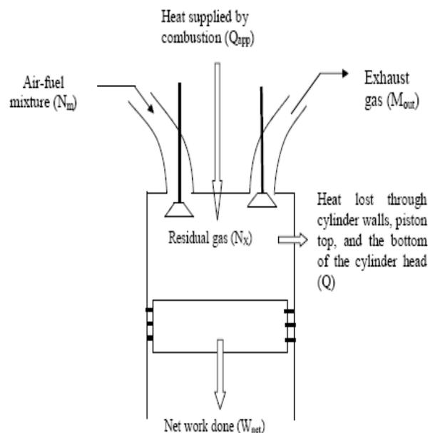
Fig 4 Schematic Diagram of Thermodynamic Modeling Process.
