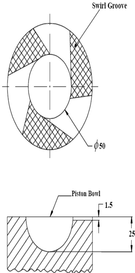
Fig 9 Geometry of Enhanced Swirl Combustion Chamber.
