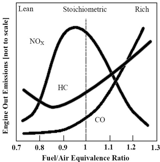
Fig 3 Effect of Air-fuel Ratio on Power, Fuel Consumption, and Emissions.
