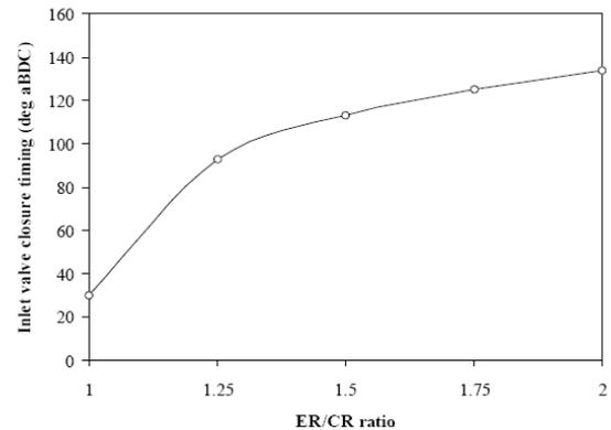
Fig 6 Variation of Intake Valve Closing Timing with ER/CR Ratio to Maintain Constant CR.
