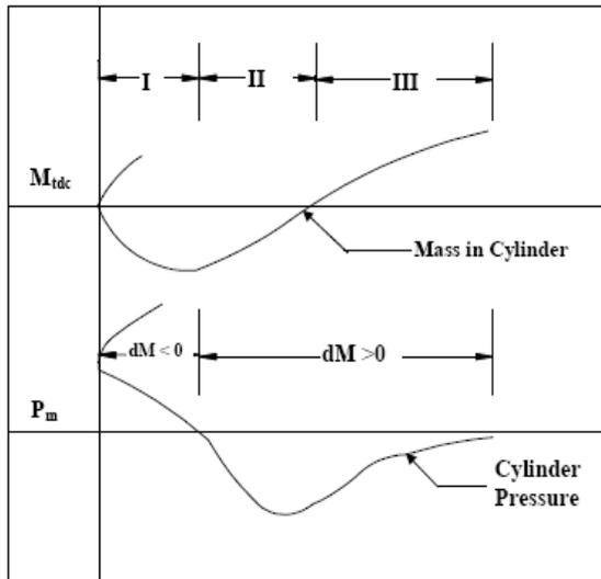
Fig 5 Particulars of Events in the Early Intake Stroke (Ganesan 1999).
