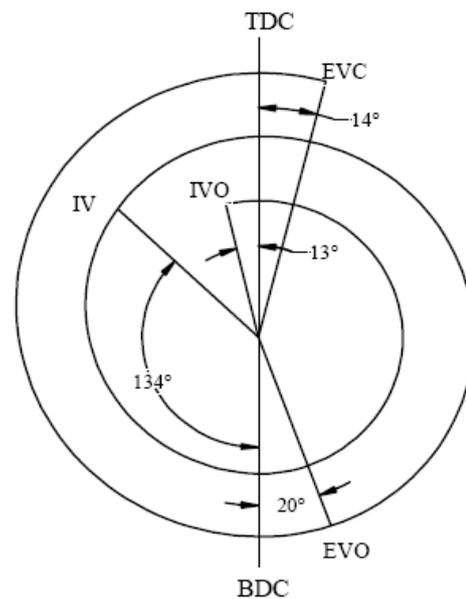
Fig 7 Valve Timing Diagram for ER/CR Ratio 2.
