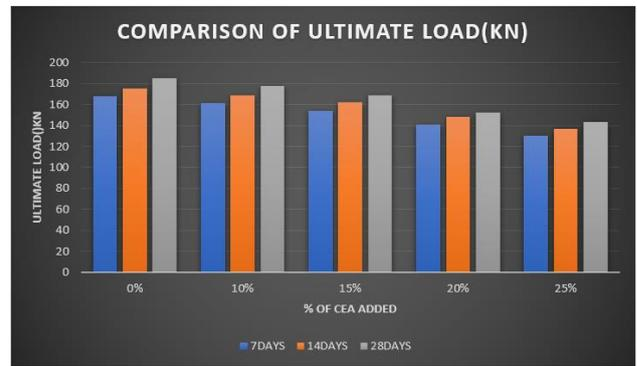
Fig. 5 Comparison Of Ultimate Load
