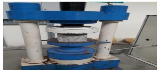
Fig 2. Compression Test Cube
