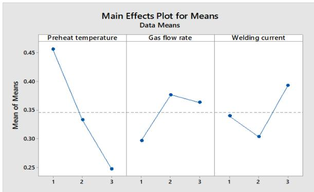
Fig. 1. Effect of welding parameters on the multi-performance characteristics
