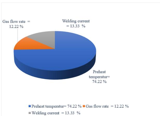
Fig 2. Percentage contribution of process parameters on tensile strength
