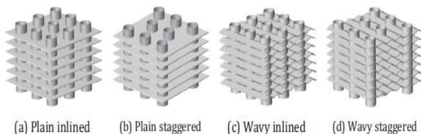
Fig. 1. Different fin and tube arrangement in plain and wavy finned-tube heat exchanger
