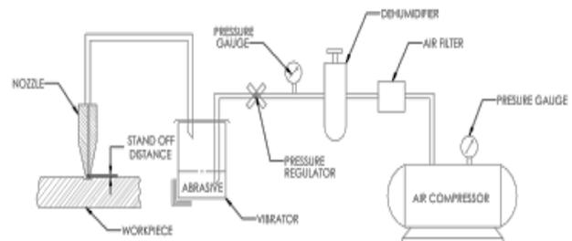
Figure 1. Layout of abrasive jet machine
