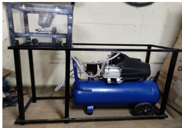
Figure 11. Complete view of abrasive jet machine
