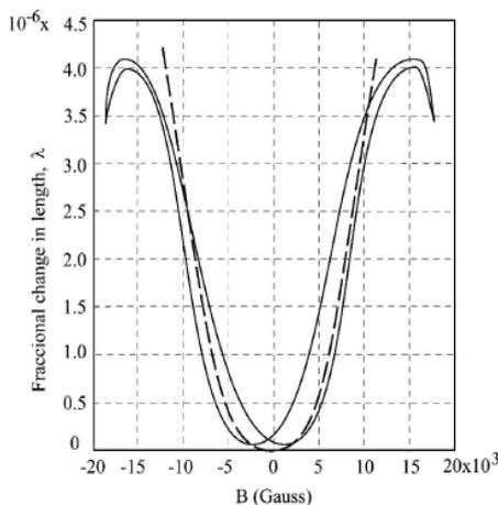
Fig 1. Iron magnetostriction as a function of induction taken from
