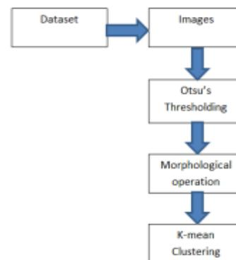
Fig.3 pre-processing and segmentation flow chart.
