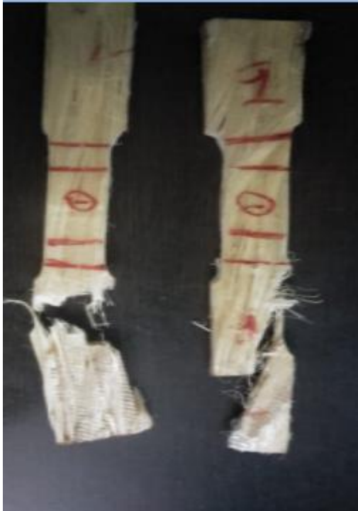
Fig.12. Tested specimen of the hemp fiber.
