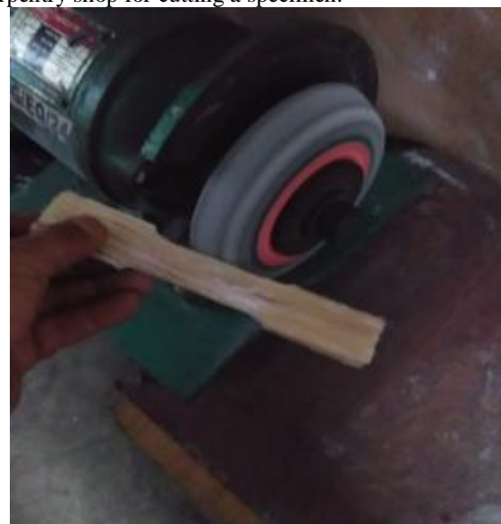
Fig .7. Preparation of the Dog-bone shape.
