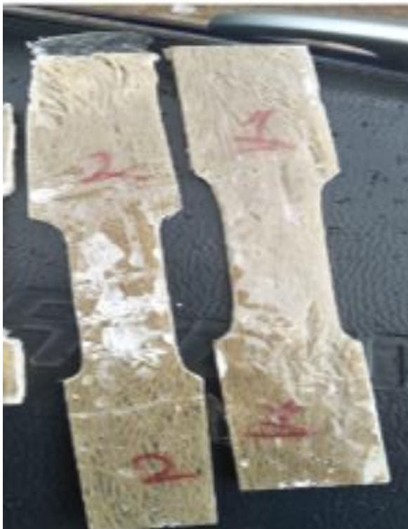
Fig .9. Dog bone shape specimen of Wool fiber.
