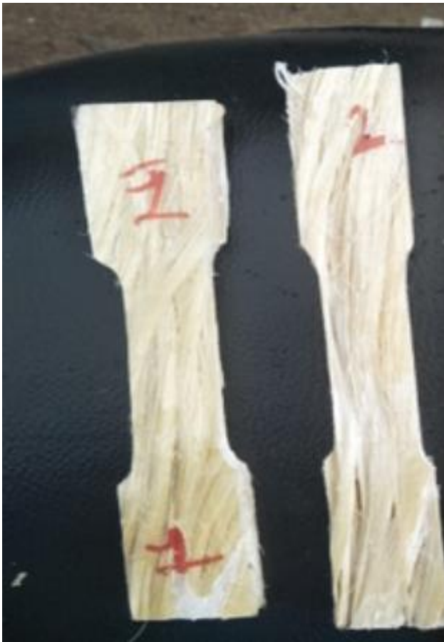
Fig .8. Dog bone shape specimen of hemp fiber.
