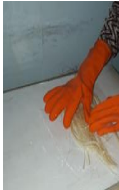
Fig. 1. Hand lay method on Teflon sheet.
