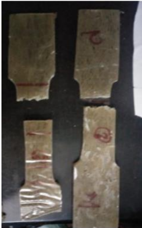
Fig.11. Tested specimens of the wool fiber.
