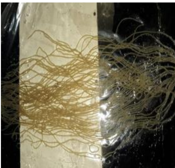
Fig .5. Laminated profile of wool natural fiber.
